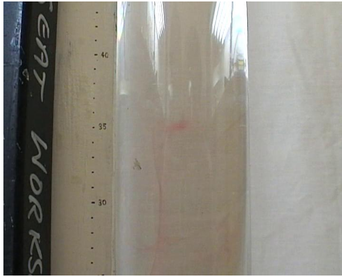
Figure C.13 One pipe upward inlet at the time, t = 1 minutes 50 seconds (2min 17sec dye injected)
