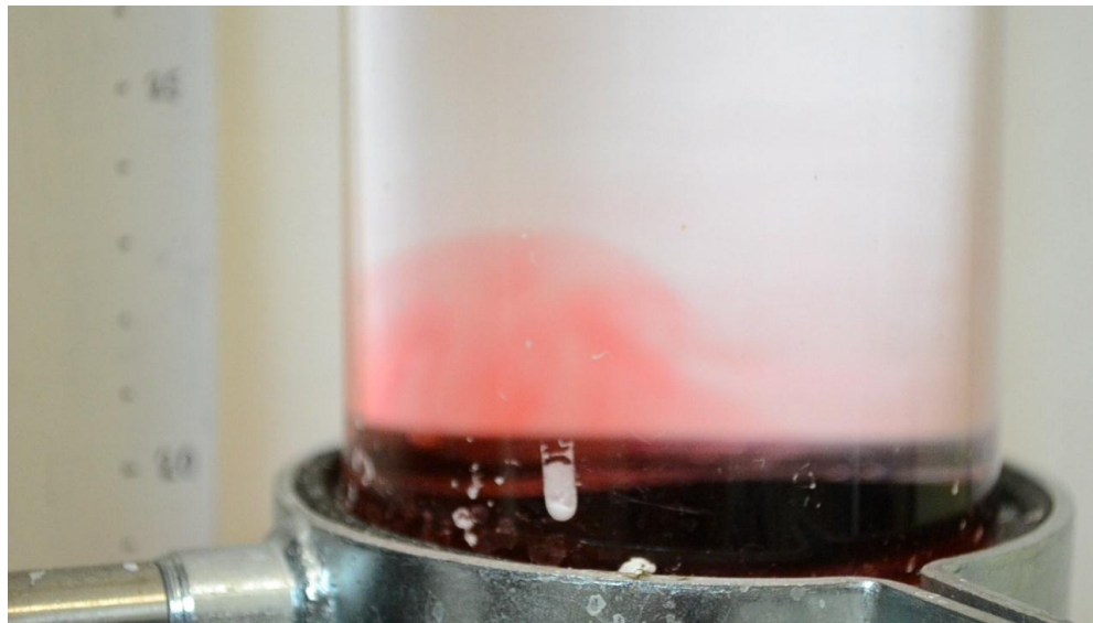
Figure C.4 16-pipes inlet at time, t = 5 minutes 22 seconds (6mins 29sec dye injected)
