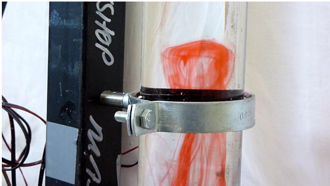
Figure C.10 One pipe upward inlet at the time, t = 1 minutes 30 seconds (2min dye injected)
