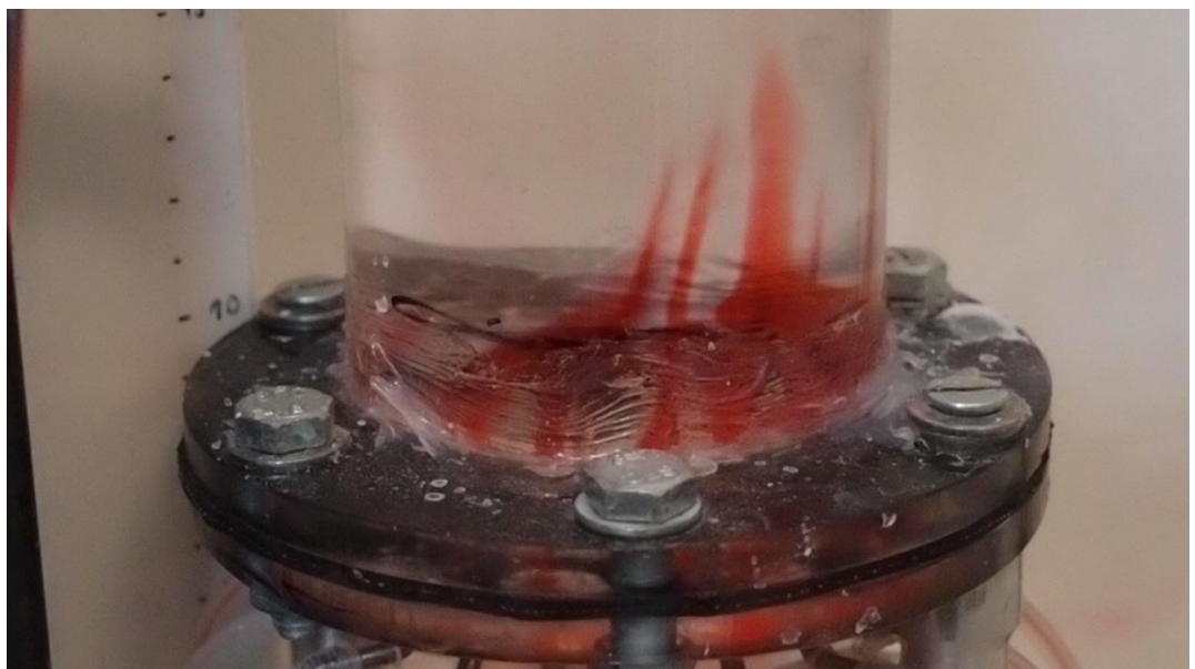
Figure C.2 16-pipes inlet at time, t = 14 seconds (30 sec dye injected)
