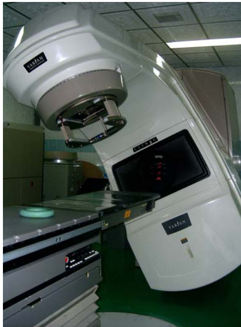
Figure 4.1 Varian 2100 C/D 6 and 10 MV for photon beam and 6, 9, 12, 16 and 20 MeV Electron beam
