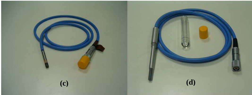
Figure 4.2 Detectors at Lopburi cancer center a) Diode p-type detector, b) Advance Markus (plane parallel) chamber, c) IC 0.3 cm 3 semiflex, d) IC 0.6 cm 3 Farmer chamber.
