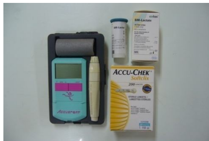
Figure 3.4 Set of instrument for determination of blood lactate concentration (Accutrend ® lactate portable lactate analyzer (Roche Mannheim, Germany)
