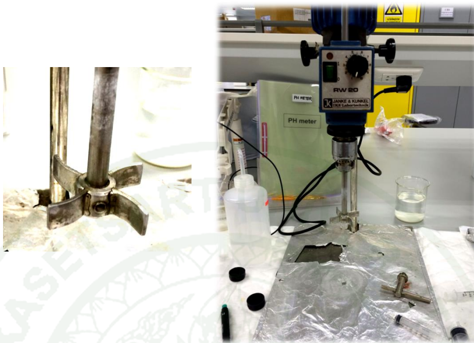
Figure 17 Blade and mechanical stir using in jar test for study flocculation ability of tapioca starch-graft-PDMC in this present work
