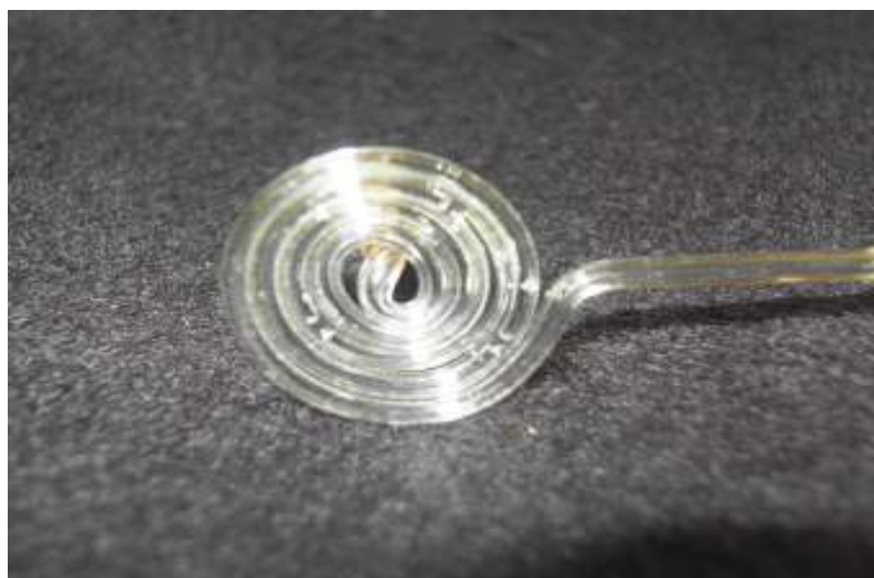
Figure 32 A flat spiral glass mixing coil for determination of Cd (II) by FI-CL
