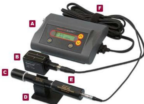
Figure 4.3 Accu-Pro™ Diagnostic Ion Chamber and kV Sensor Components
