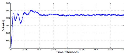
Figure 8 Simulation result for DC-Link voltage
