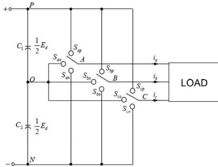
Figure 4 Simplified mode of three-level inverter
