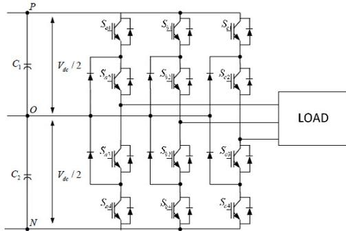
Figure 3 Main circuit of three-level inverter.
