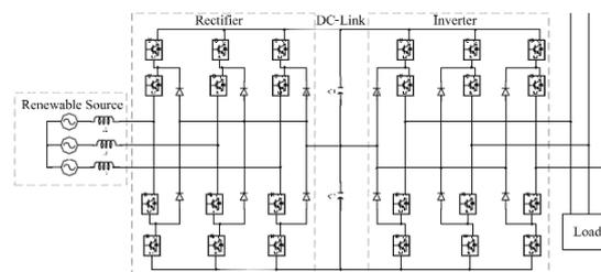
*Figure 1 Main circuit of three-level back-to-back converter.*
