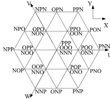
Figure 5 Voltage space vector diagram of three-level inverter.
