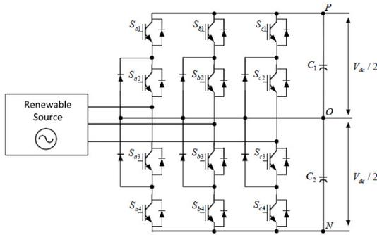
Figure 2 Main circuit of three-level rectifier.
