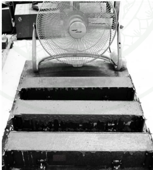
Figure 9 Restrained shrinkage cracking test setup.
