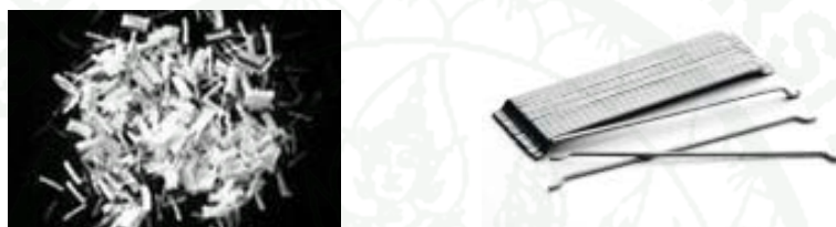
Figure 7 Fibers used in this study, polyvinyl alcohol (L) and steel (R)
