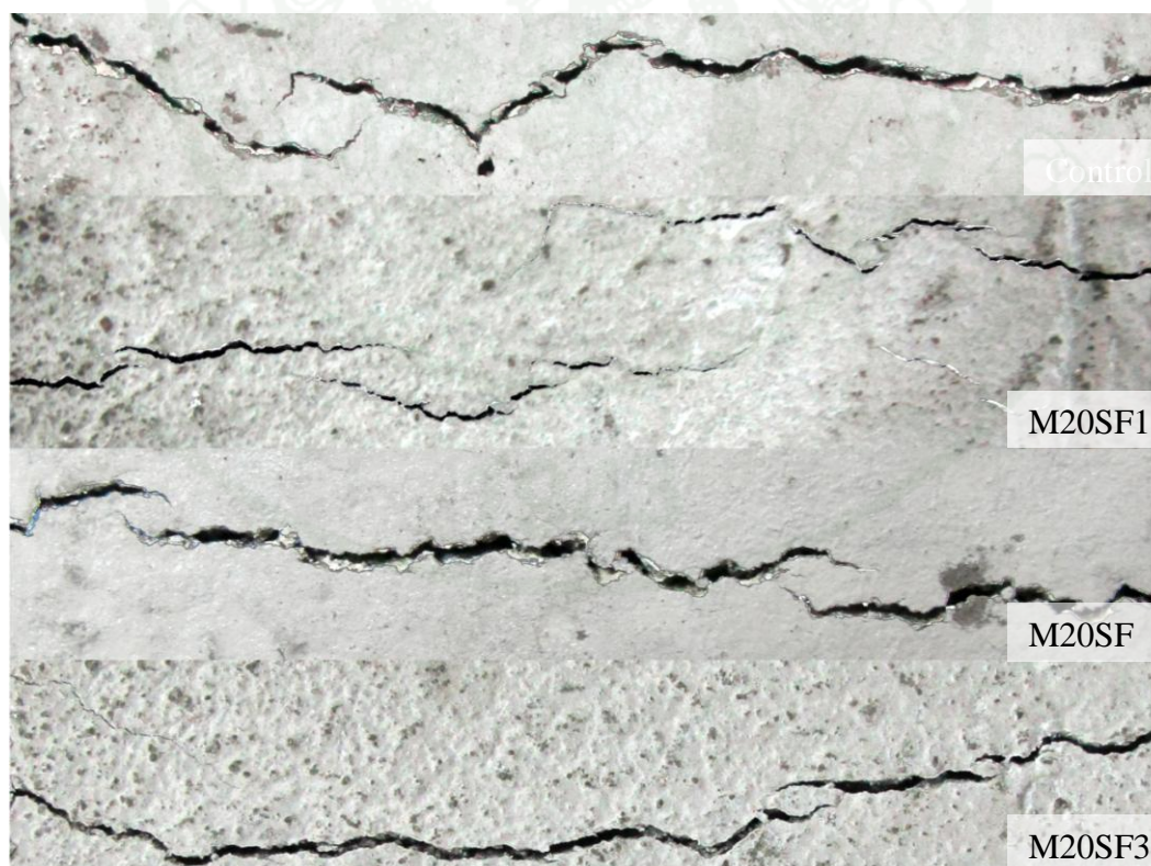
Appendix Figure 8 Cracked specimens, M30- Steel fiber concrete
