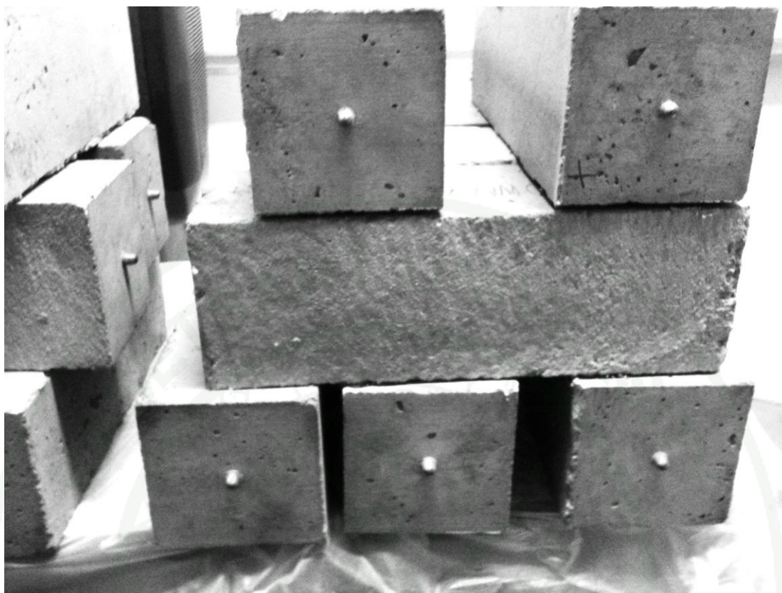
Appendix Figure 11 Free shrinkage specimens after unmolding
