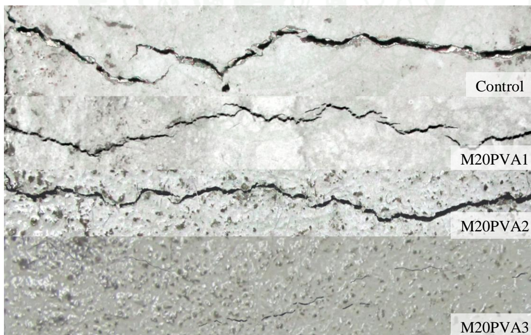
Appendix Figure 6 Cracked specimens, M30- PVA fiber concrete
