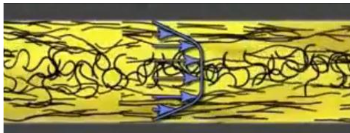
Figure 2.6 Molecular orientation through the cross section [12]
