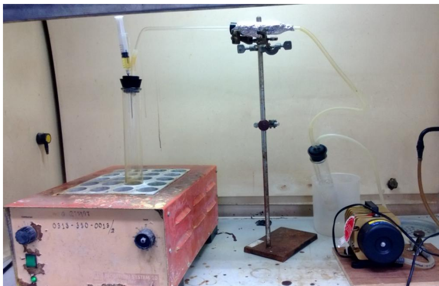
Figure 3.3 Dropping oil combustion and smoke collection system
