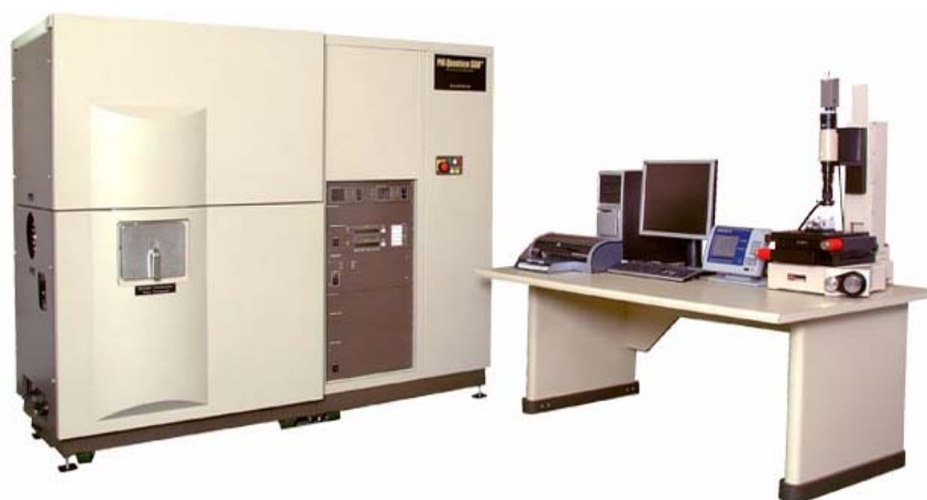
Figure 3.8 X-ray photoelectron spectroscopic (PHI Quantera SXM).
