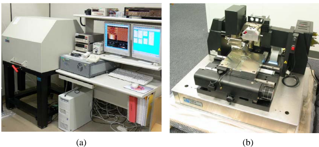
Figure 3.7 Atomic force microscope (AFM) in a tapping mode, Digital Instruments Veeco, Dimension 5000 (a) AFM and display part (b).
