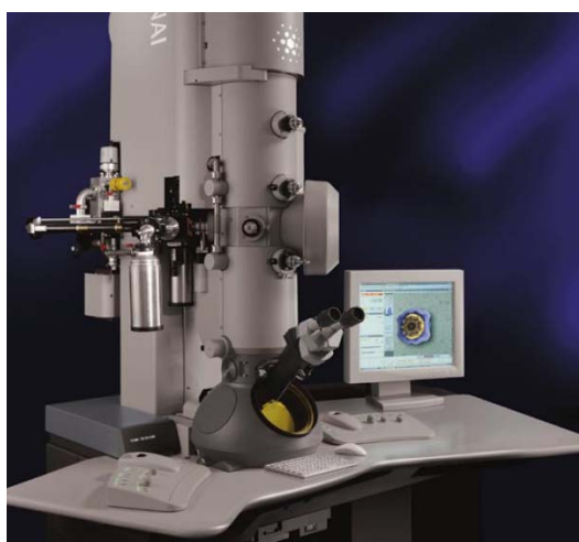
Figure 3.9 Transmission electron microscopy (TEM) working at 200 kV, FEI, Tenai TM G 2 20.
