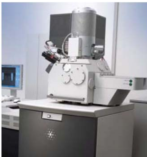
Figure 3.10 Focus ion beam(FEI, Strata TM 400 Dual Beam TM ) working at 2-30 kV.
