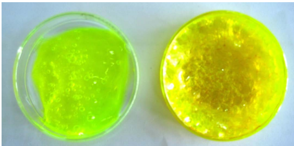
Figure 4.3 PPV (right) product after elimination of the sulfonium group (left)
