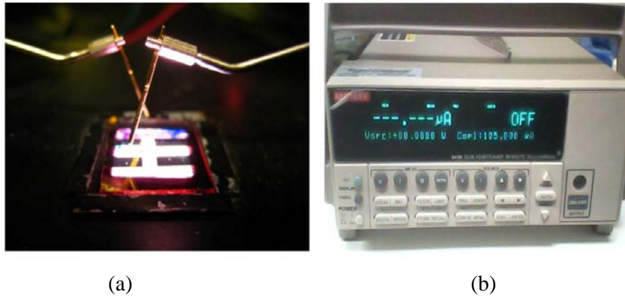
Figure 3.16 Images of (a) J - V measurement and (b) Keithley 6430 digital multimeter
