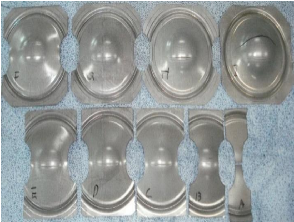
Figure 3.24 Deformed specimens after failure in the Nakazima test.
