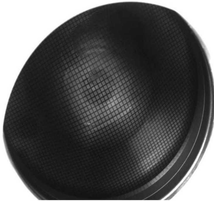
Figure 3.23 Thickness distribution and localized necking area on the deformed specimen at localized state during test
