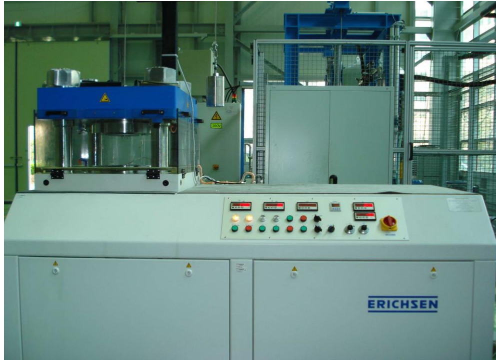
Figure 3.6 Erichsen bulge/FLC tester model 161
