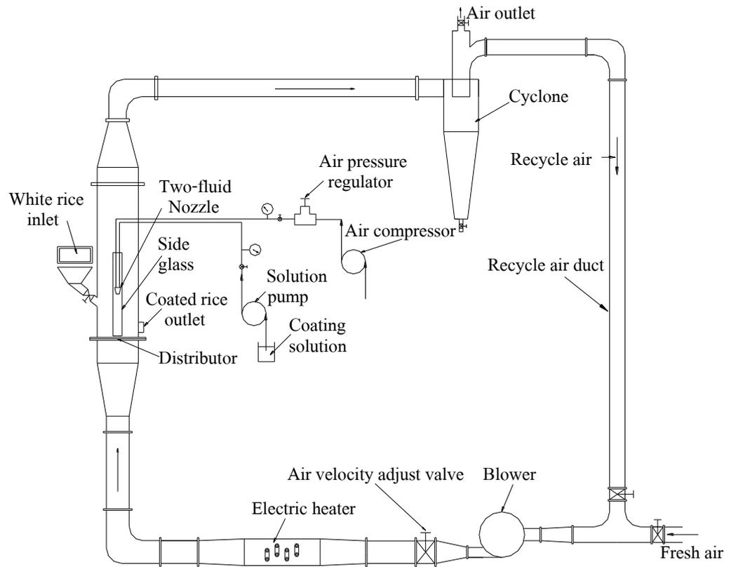
**Figure 3.1** A schematic diagram of top-spray fluidized bed apparatus
