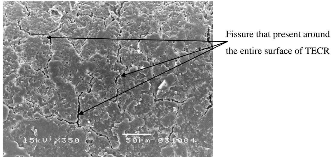
**Figure 3.5** Scanning electron micrograph of fissuring feature of TECR at coating condition of inlet air temperature of 60 °C and spray rate of coating solution of 34 mL/min
