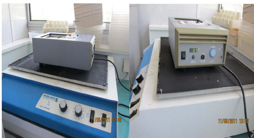
Thermostatically controlled shaker (Bioblock Scientific Ping-Pong 74582)
