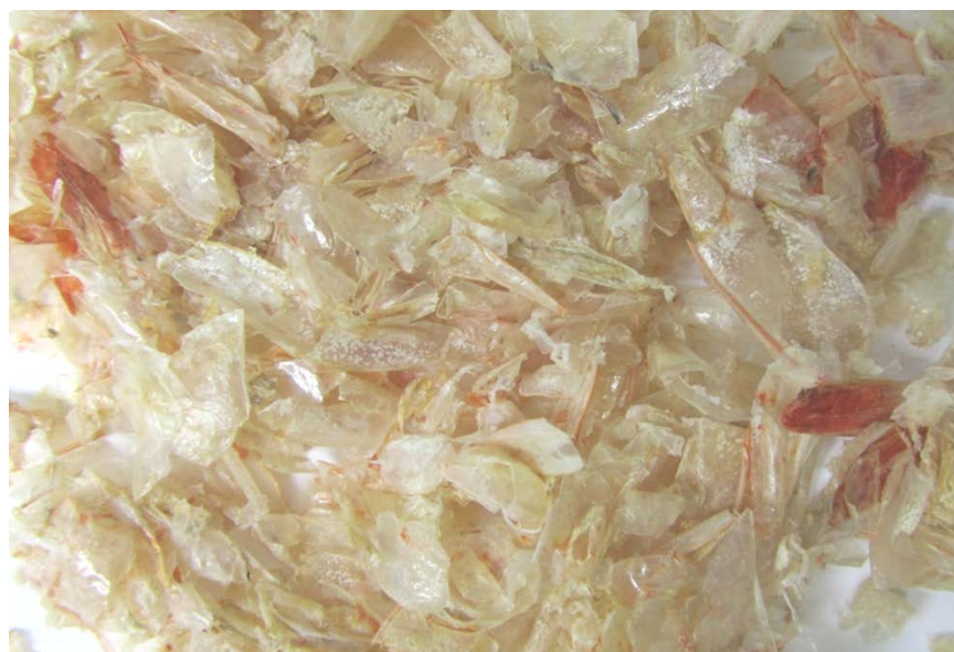
Figure 4.27 Decalcified shrimp shells by fermentation with isolate L7 using whey as carbon source
