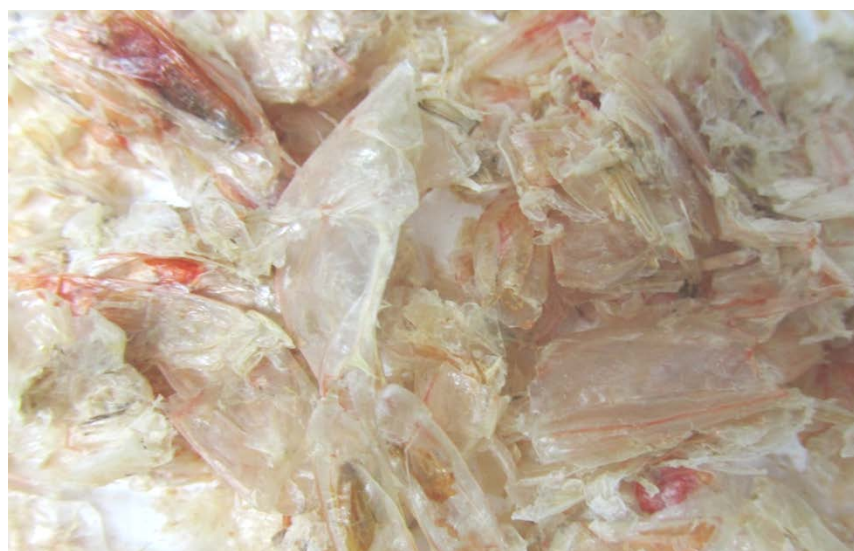
Figure 4.25 Decalcified shrimp shells by fermentation with isolate L7 using a sucrose as carbon source
