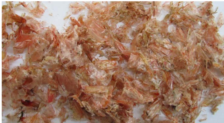
Figure 4.21 Decalcified shrimp shells with lactic acid fermentation for 2 days with 30% inoculums and 20% glucose (w/w shrimp shell weight)
