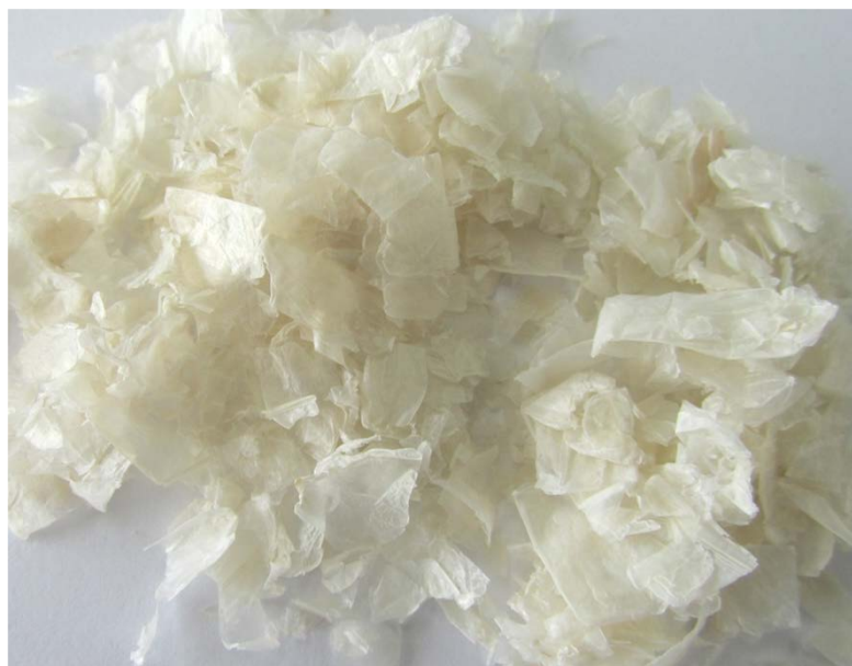
Figure 4.52 Chitosan flakes obtained from deacetylation of biologically purified chitin at 121°C for 5 h
