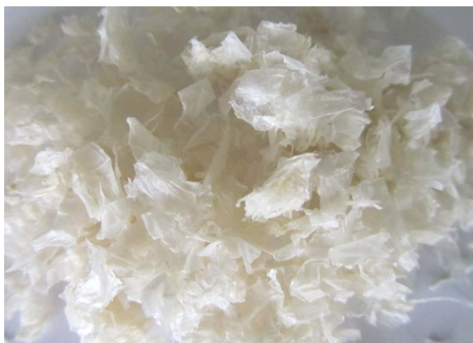
Figure 4.47 Chitosan flakes obtained from deacetylation of chemically processed chitin at 121^\circ\text{C} for 5 h
