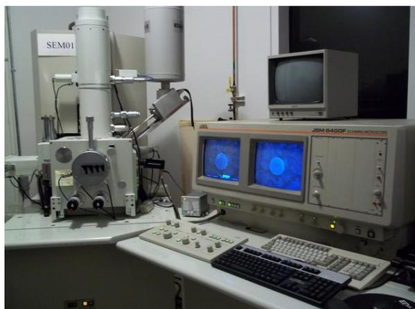
Figure 3.3 General view of the scanning electron microscope integrated with the energy dispersive X-ray spectrometer (SEM-EDS: JEOL, JSM-6400, Link ISIS-300).
