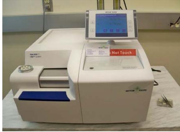
Figure 3.4 General view of the “Mettler-Toledo” TGA/DSC1 thermogravimetric analyzer.
