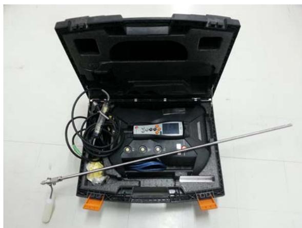
Figure 3.5 General view of “Testo-350” gas analyzer (Testo, Germany).
