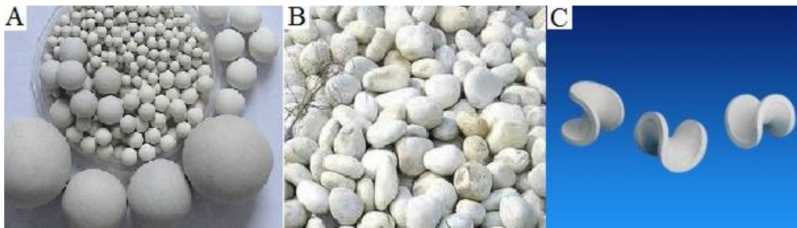
Figure 2.3 Discrete element: A) Ceramic balls, and B) Ceramic pebbles, and C) Ceramic saddles.
