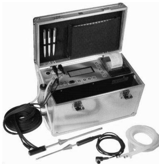
Figure A.8 Visit-01L exhausts gas analyzer.
