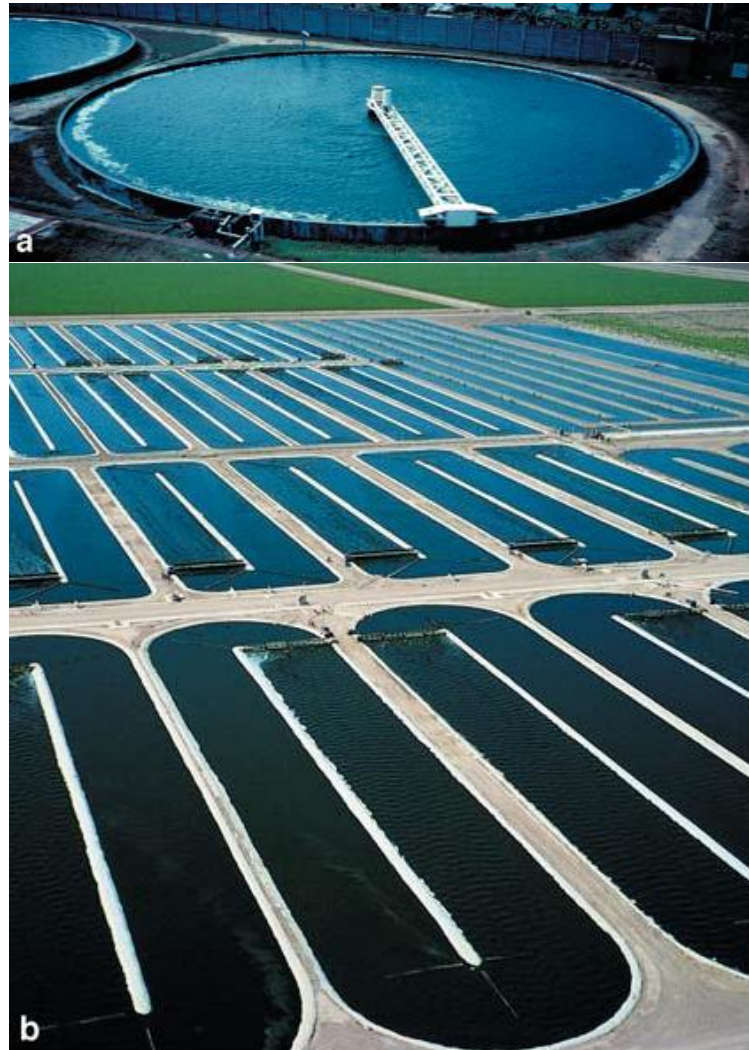
Figure 2.1 (a) Center-pivot pond used for the cultivation of Chlorella in Taiwan (b) Raceway ponds used for the culture of Spirulina by Microbio Inc. at Calipatria, California [4].
