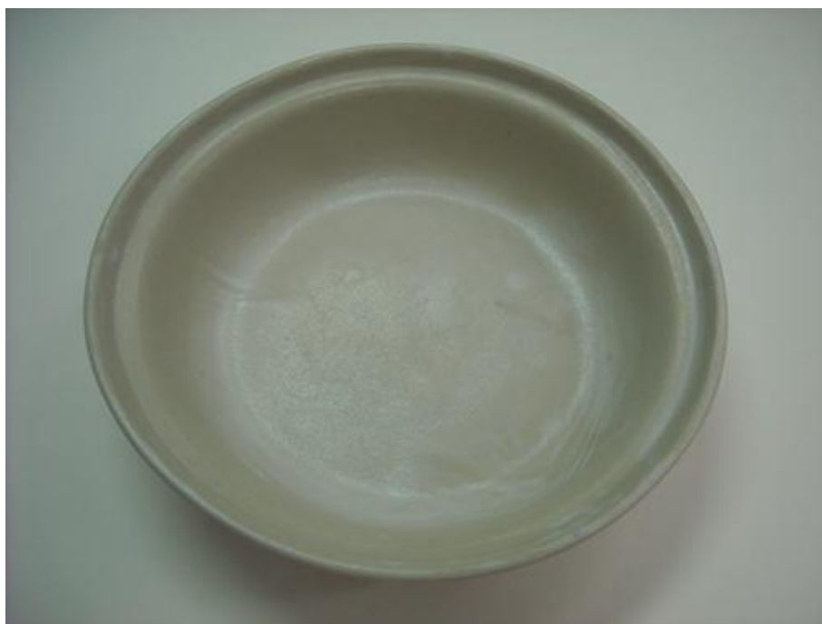
Figure 5.23 The prototype S7-6-15 after pass thermal shock resistance test at 290°C for 5 times
