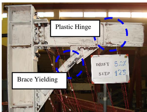
**Figure 2.20** Plastic Hinging and Brace Yielding in Test Specimen at 5% Story Drift.
