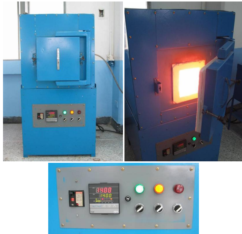
Figure 3.3 High-temperature heat treatment furnace
