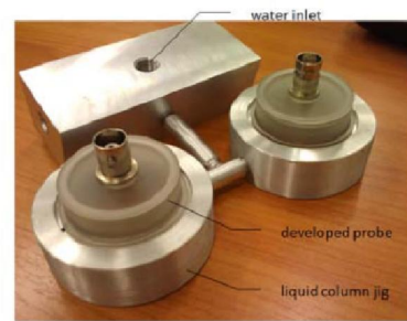
Figure 9. Designed jig with a dual probe support.
