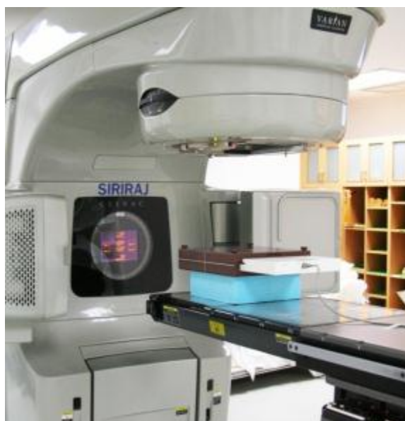
Figure 4.17 2D dose distribution IMRT verification using MapCHECK2 TM and MapPHAN TM
