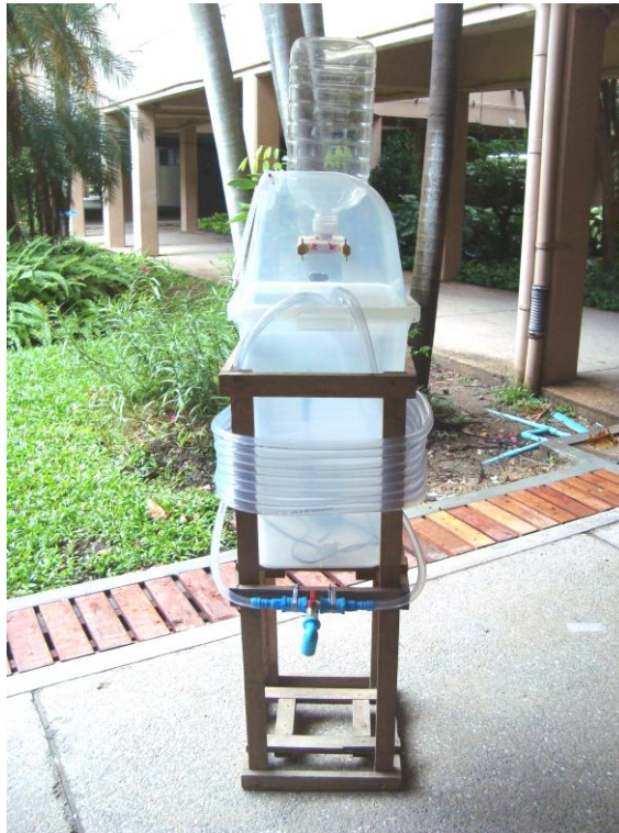
Figure 3.2 A tubular photo-bioreactor in this study
