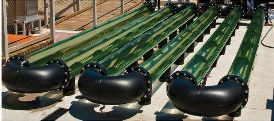
**Figure 2.7** Tubular photobioreactor
