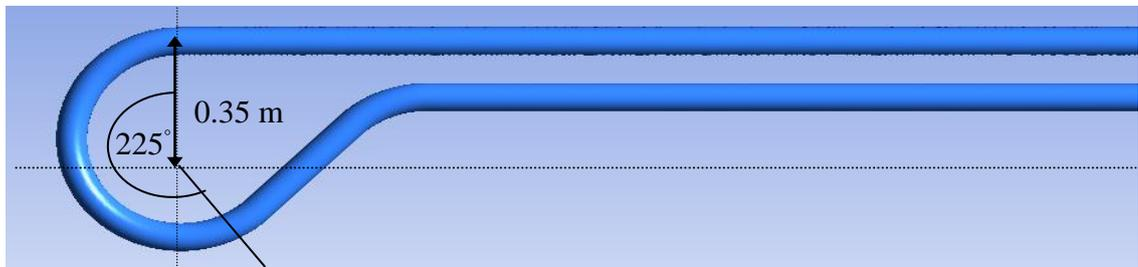
**Figure A.6** Type 4 of U-bend configuration
