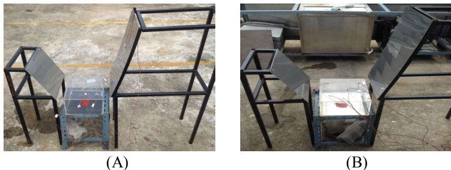
Figure 2. (A) Set 1 the system with a metal plate coated with \text{TiO}_2 (B) Set 2 the system with a metal plate without \text{TiO}_2 .
