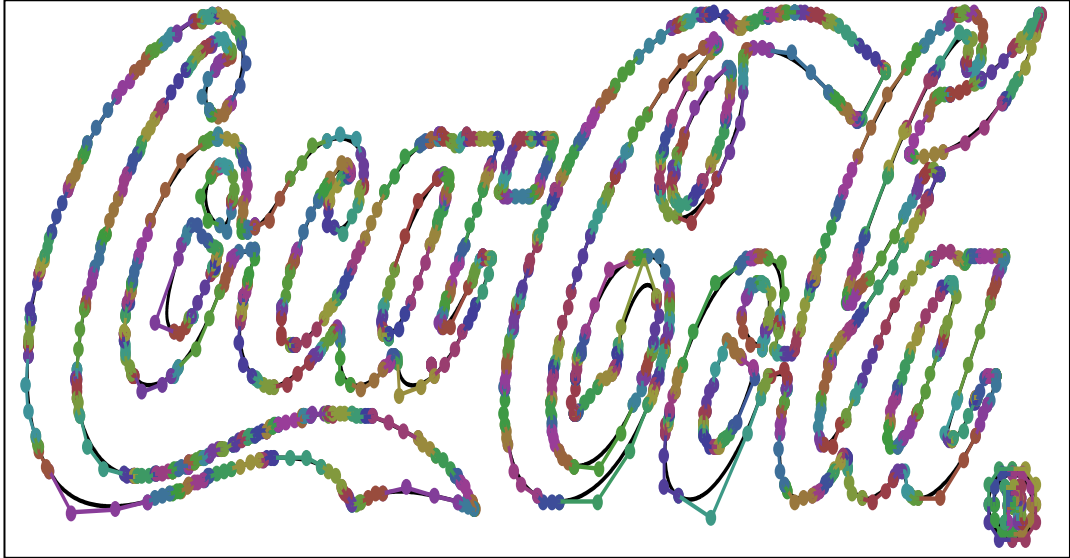
Figure 5 Input of Conversion is displayed as Approximation (Bézier) curve with its control points.
