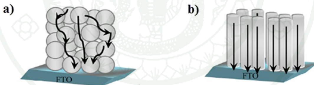
Figure 5 The diagrams of electron mobilization in TiO 2 medium. a) a random pathway in the colloidal film. b) a direct pathway in the 1-D nanostructured TiO 2 film.
