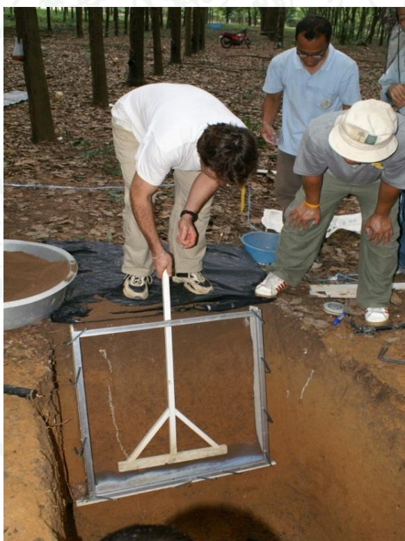
Figure 6 Horizontal and vertical rhizotron installation in the study plot
