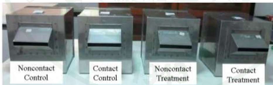
Figure 12 Excito-repellency test system showing the four chambers aligned in sequence for each trial run, one pair as contact and matched control, the other set as non-contact and control chamber.
