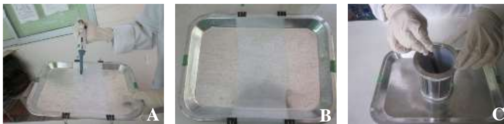
Figure 4 Net impregnation, (A) Using a micropipette evenly spread solution on the net, (B) The treated net allowed to air dry for 15 min, (C) After 15 min, a treated net was rolled inside the treatment drum
