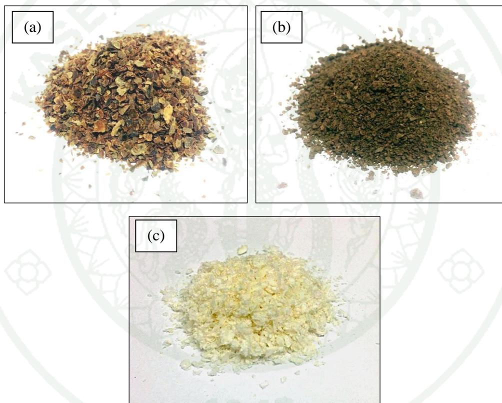
**Figure 12** Photographs of mango peel; untreated fibers (a), steam-exploded fibers (b) and bleached fibers (c).
