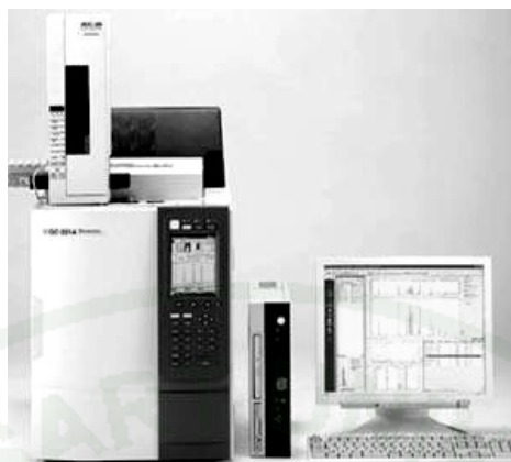
Figure 25 Shimadzu gas chromatograph (GC-2014) equipped with thermal conductivity detector (TCD) and chromatopac data processor.
