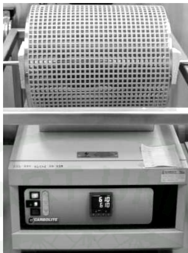
Figure 23 The reactor of methane cracking reaction equipped with the electric heater (Carbolite tube furnace).
