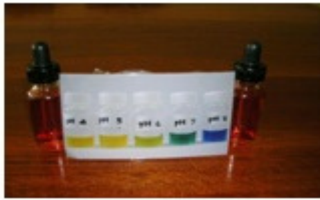
Locally made pH test kit to substitute imported pH meter
