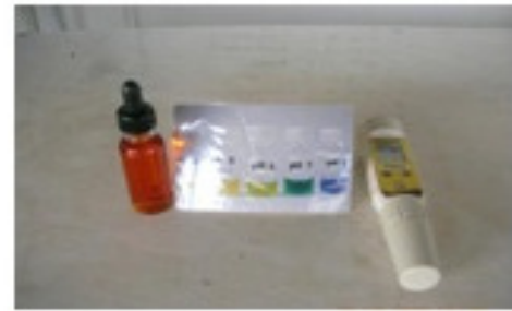
Locally made pH test kit to substitute imported pH meter
