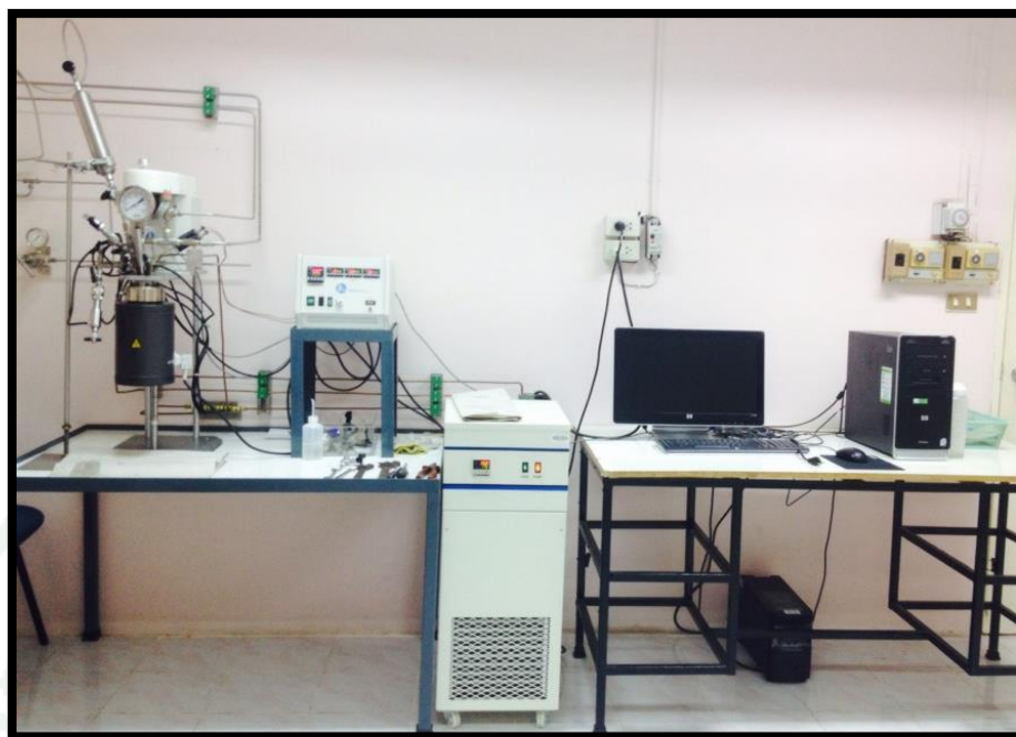
Appendix Figure F1 Overall of high temperature and pressure batch reactor
