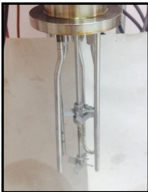
Appendix Figure F3 Four- blade impeller, cooling tube, fine filter thermocouple and pressure sensor
