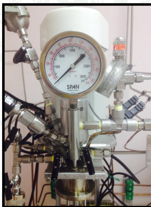
Appendix Figure F4 Head assembly; gas inlet valve and gas release valve
