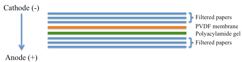
Appendix Figure A1 The orientation of PVDF membrane and polyacrylamide gel.
