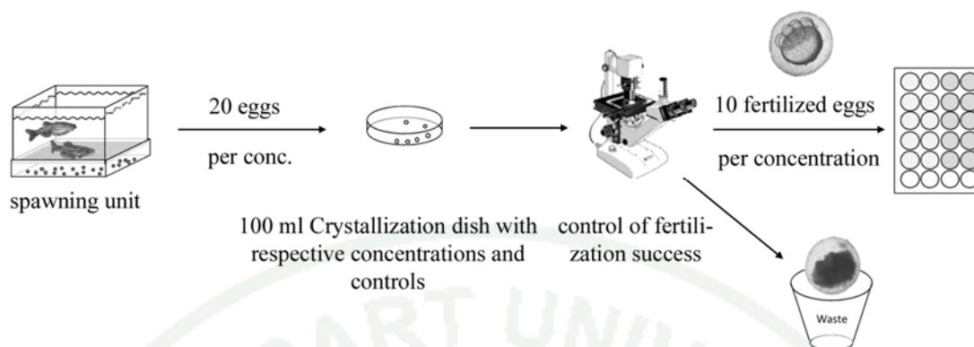
**Figure 7** Scheme of the FET test procedure (from left to right): collection of the eggs, pre-exposure of the eggs immediately after fertilization in crystallization dishes, selection of fertilized eggs with an inverted microscope or binocular and distribution of the fertilized eggs into prepared 24-well microtiter plates
