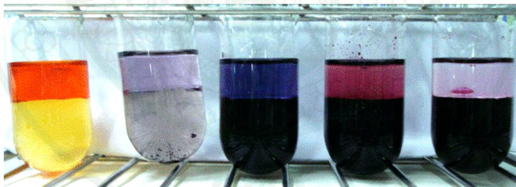
**Figure 23** Characteristics of solutions between octanol and aqueous phases of 5 azo dyes after shaking for 1 hour with shaking incubator at 25±1°C. Above and below phases are octanol and aqueous phases, respectively.
