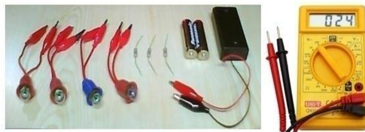
Figure 3.2 Basic electric components used in the activities: light bulbs with holder and crocodile clip, resistors, battery and holder, and digital multi-meter
