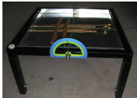
Figure 3.2: Instrument for ankle joint position sense testing.
