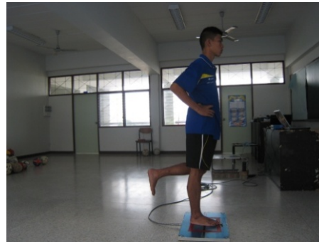
Figure 3.3: Center of pressure test in single-leg-stance position on a force platform.
