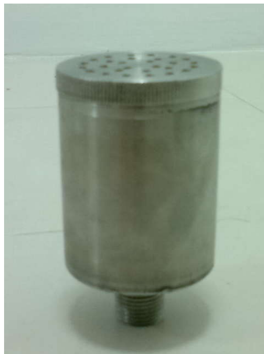
Figure 3.8 Schematic diagram of the single perforated tube silencer.
