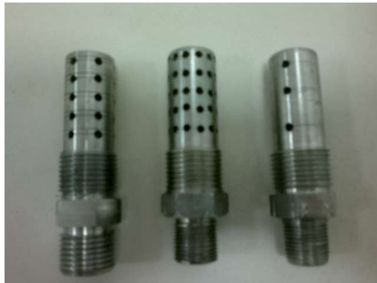
Figure 3.6 Perforated tubes in the single perforated tube silencer (from the left, A, B and C)
