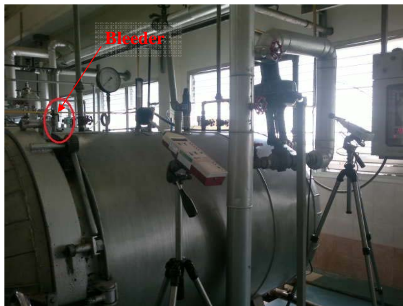
Figure 3.11 The points of sound pressure level before install silencer for noise reduction testing from retort.
