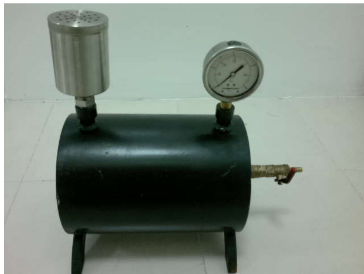
Figure A-5 The test sound pressure level from air pressure while install silencer
