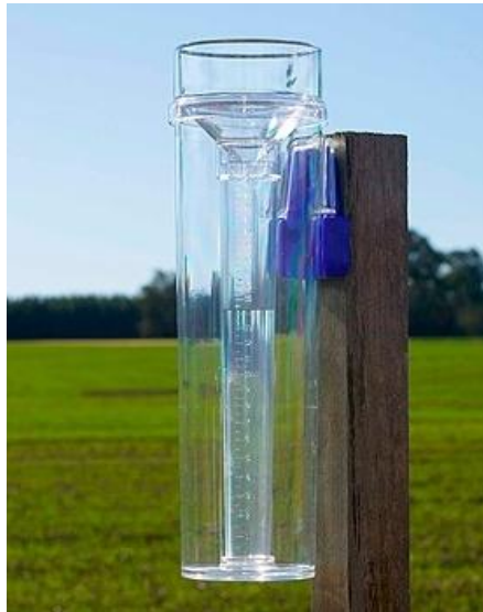
Figure 4.4 Rain gauge used to gather and measure the amount of liquid precipitation over a set period of time
