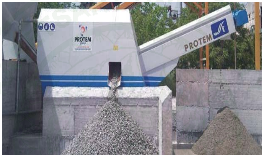
Figure 5 Reclaimer system for concrete waste
