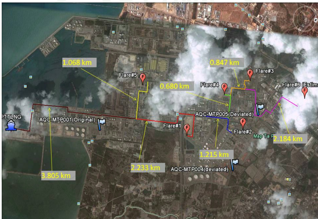
Figure 35 Route and distance of pipeline between waste gas source and LNG receiving terminal.
