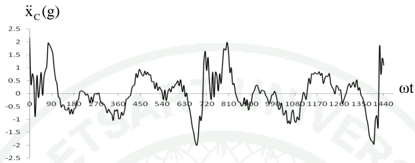
Figure 27 The engine acceleration at point C in x direction ( \ddot{x}_c )
