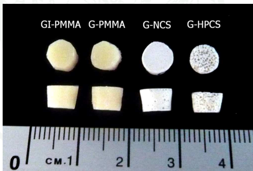
Figure 14 The beads were presented in each group in top and side views. Beads were arranged from left to right in the following order: GI-PMMA, G-PMMA, G-NCS and G-HPCS, respectively. GI-PMMA and G-PMMA beads had no visible pores on the surface while G-NCS beads had little pore numbers on the surface. Numerous visible pores were found on the surface of G-HPCS in both top and side views.
