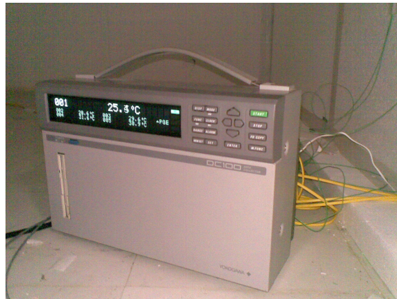
(b) Data collector (Yokogawa, DC-100)
