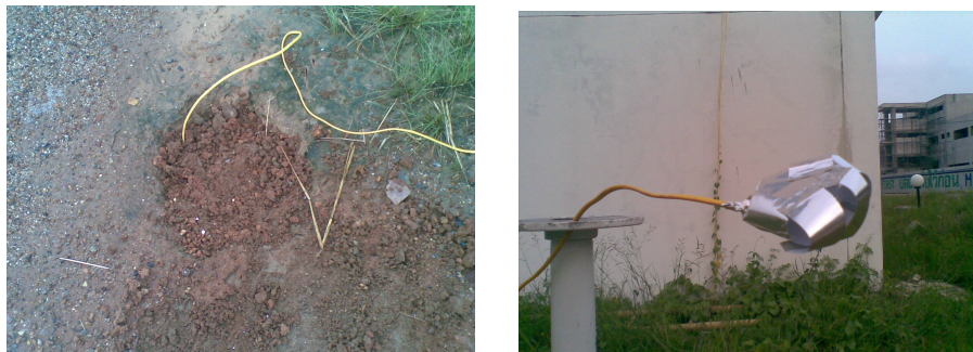
(c) Thermocouple at ground surface and on the outside building
