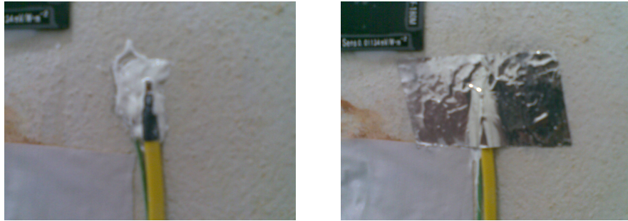
(a) Thermocouple installation on the test wall.
