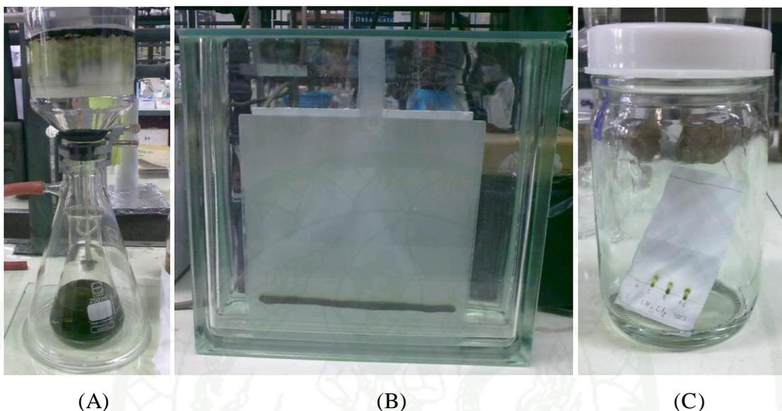
**Figure 14** (A) Quick Column Chromatography, (B) Preparative Thin Layer Chromatography and (C) Thin Layer Chromatography
