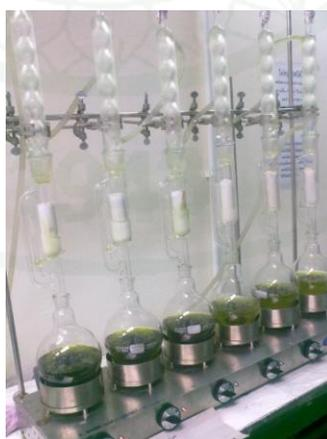
**Figure 10** *W. trilobata* extraction by using Soxhlet's apparatus
