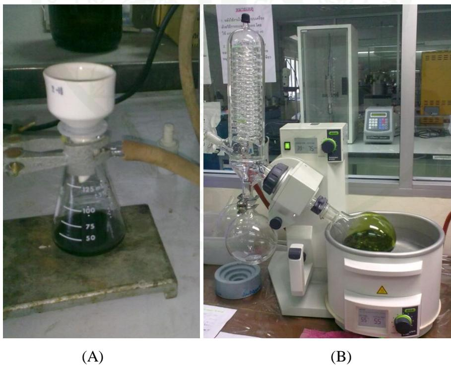
**Figure 12** Vacuum pump filter (A) and Evaporation (B)
