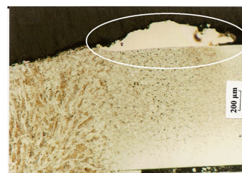
Figure 12. Accumulation of Zn on the weld surface, sample B2
