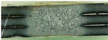
Figure 4. Weld macrostructure of A4 sample, diameter of weld nugget d = \varnothing 5 \text{ mm}
