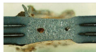
Figure 14. Macrostructure of the weld, sample B4
