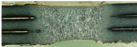
Figure 3. Weld macrostructure of A2 sample, diameter of weld nugget d = \varnothing 4.3 \text{ mm}
