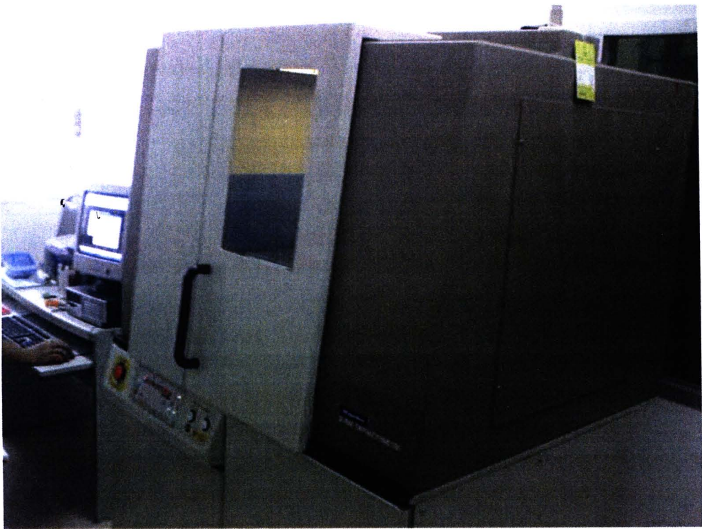
Figure 2.11 An illustration of the Rigaku Rint 2000 X-ray diffractometer
